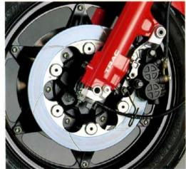
Dual floating mount front discs with dual-piston calipers and sintered metal pads.
