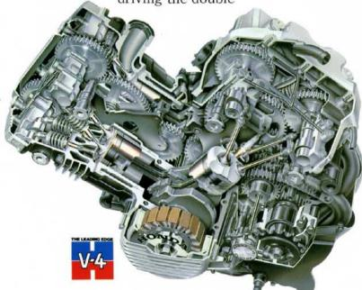
overhead camshafts. The idler gear and camshaft @ gears are of the split type with coil springs to maintain constant gear-to-gear contact and ensure quiet running. The engine runs a phenomenal 10.7:1 compression ratio boosting power output. A special combustion chamber and squish band design makes this possible without detonation even on unleaded gas while an efficient oil cooler keeps it running cool. Power is delivered by a hydraulically actuated clutch with a ride-smoothing one-way mechanism.
