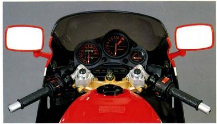
Ergonomic control center with rubber mounted instruments and racer-type large dial electronic tachometer. Compact switch design puts everything at your fingertips.
